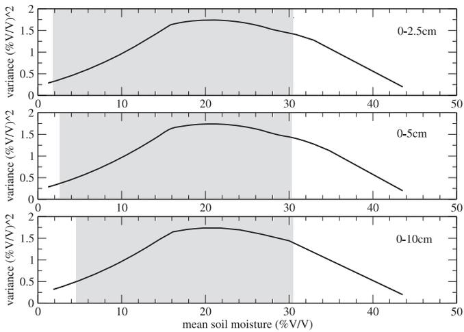
FIGURE 3. The Plots of Mean Soil Moisture vs. Variance of Soil Moisture for Owe *et al.*'s Case in Three Surface Horizons (0-2.5, 0-5, and 0-10 cm). The observed dynamic range of mean soil moisture by Owe *et al.* is also shown as the shaded area on each plot.
