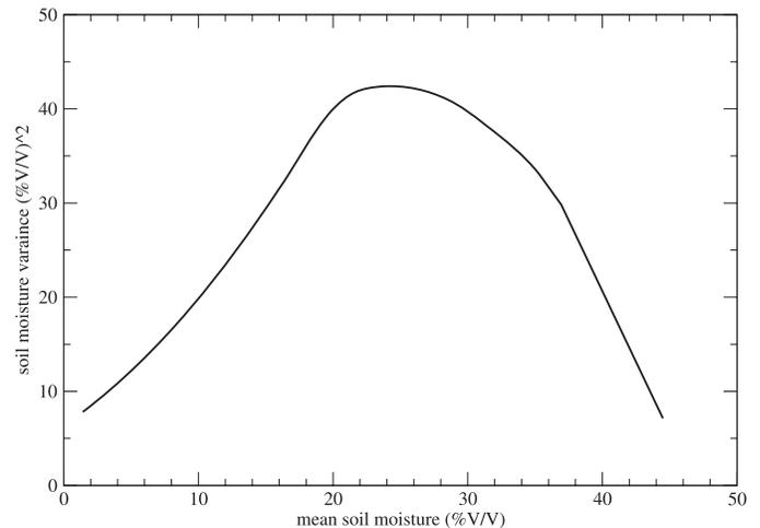
FIGURE 2. The Plot of Mean Soil Moisture *vs.* Variance of Soil Moisture for an Idealized Case. The variance of soil moisture reaches its maximum as mean soil moisture is equal to 24.5 (% v/v).
