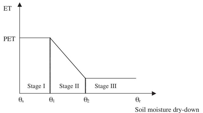
FIGURE 1. (a) The Three Stages of the Actual Evaporation. (b) The actual evaporation rate as a function of soil moisture and the potential evaporation rate in the three stages during a soil dry-down process.
