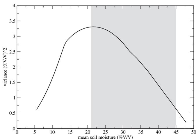
FIGURE 5. The Plot of Mean Soil Moisture *vs.* Variance of Soil Moisture for Hupet and Vanclooster's Case. The observed dynamic range of mean soil moisture by Hupet and Vanclooster is also shown as the shaded area on the plot.
